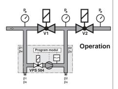
Idle state: Valves 1 and 2 are closed. Pressure build-up: The internal motor pump increases the gas pressure in the test section by approx. 20 mbar compared to the input-side pressure applied to valve V1.
