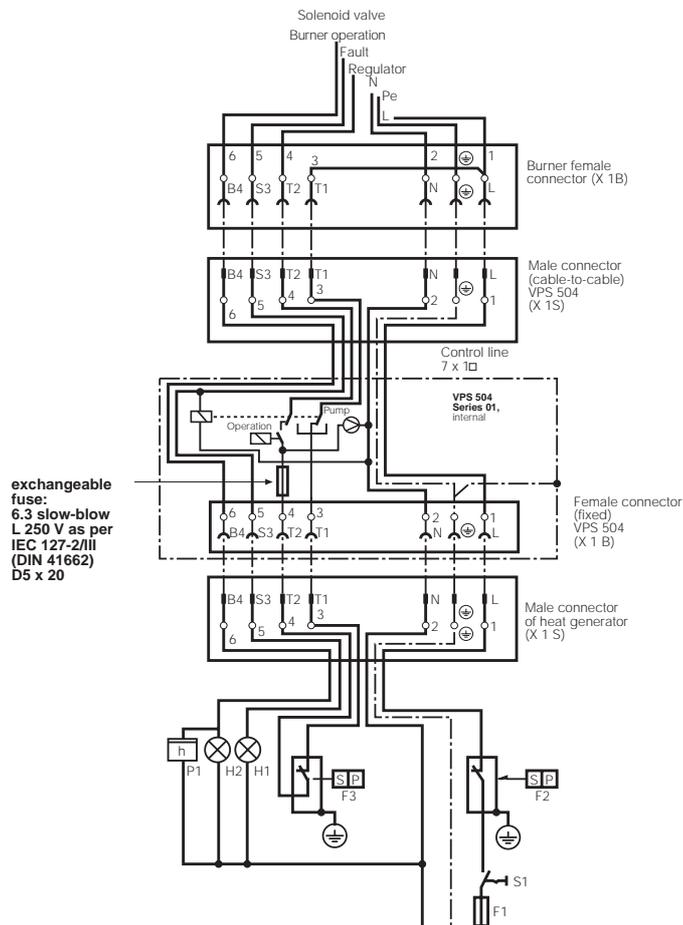
**⚠ Only the fault signal coming from the automatic burner control of the burner may be connected to connection S3. If you do not observe this instruction, persons may be injured or objects may be damaged. Therefore, strictly keep to this instruction.**
