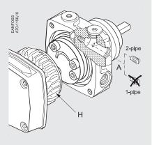
2-pipe: Screw (A) fitted 1-pipe: Screw (A) removed In 2-pipe systems the excess oil is led back to the return outlet (R). In 1-pipe systems with plugged return outlet (R) and removed bypass screw (A), the oil is returned internally to the gear set (see details in below figure). When the pump is stopped the pressure drops and the spring force in the pressure regulator will move the piston until it seats and the oil flow is shut off effectively.
